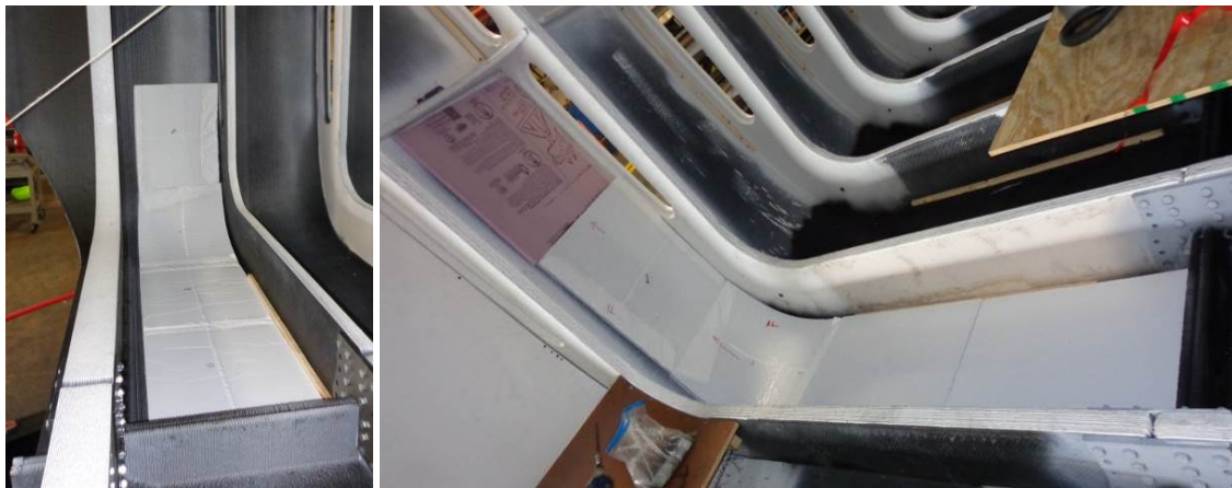
Figure 9 MAI inserted into the 3D printed rings during assembly.
