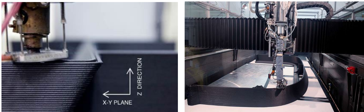
Fig. (5): Left: Printing ABS layers; Right: Printing one of the AMIE rings on the BAAM.
