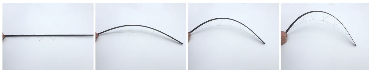
Figure 8: CFRP plate actuation of the scale model prototype
