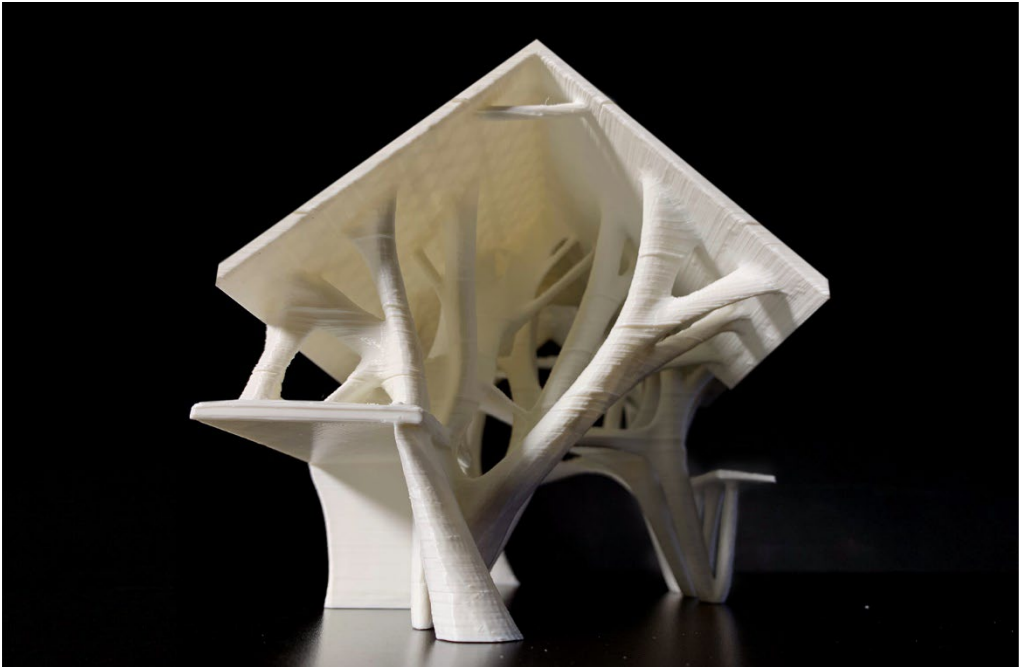
Figure 1: 3d-printed model of topologically optimized U-House prototype.
